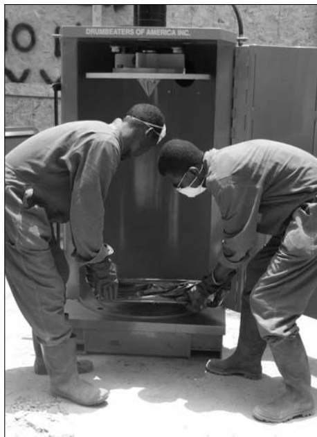
Metal pesticide drums are crushed after use, Mauritania
