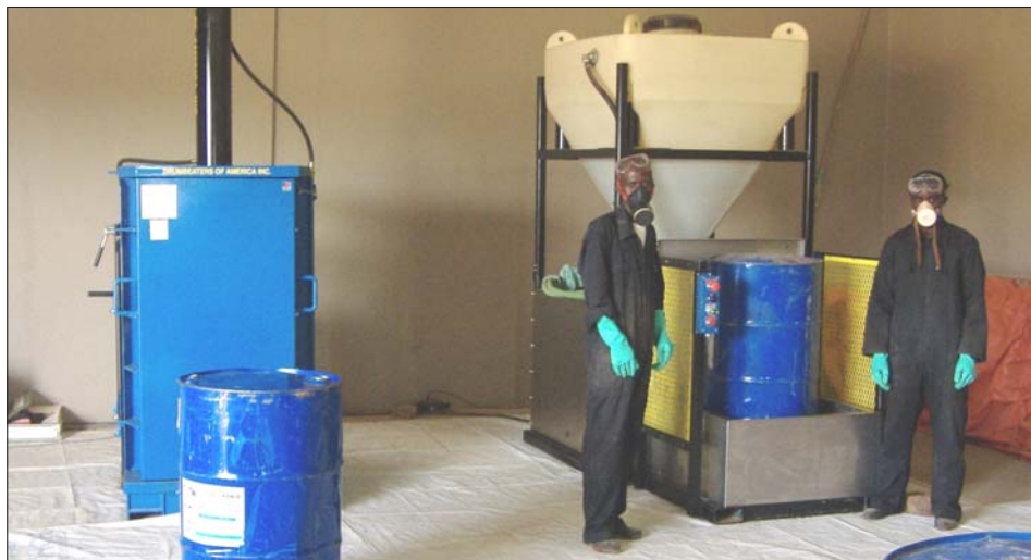
Press installed in Mali to make empty metal pesticides containers unusable Photo: Abou Thiam
